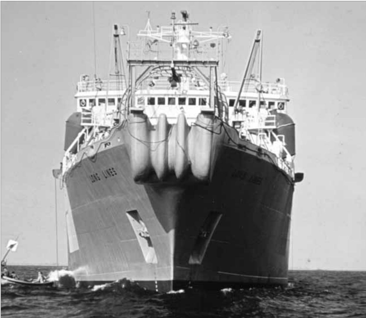
Figure 1.6: CS Long Lines which, together with cable ships from France and the United Kingdom, laid the first trans-Atlantic fibre-optic cable (TAT-8). Source: AT&T Inc.
